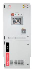
The EasyExhaust<sup>™</sup> Pyrolizer/Wet Scrubber will first thermally decompose/oxidize gases in a furnace, then pass the gases through a water spray packed tower to wet scrub, remove particles and cool the exhaust gases prior to exiting the system.
