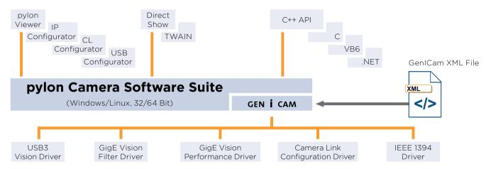
The architecture of the pylon Camera Software Suite is based on GenlCam Technology, which offers you easy access to the newest camera models and the latest features. Changes to an existing camera device in your application essentially become a plug-and-play process.
