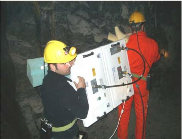
RIS Configuration with 80 MHz Shielded Antenna- Acquisition Phase
