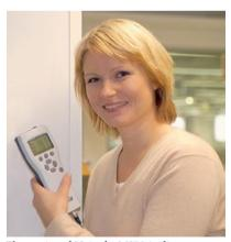
The optional Vaisala MI70 indicator can be used as a display for the DMT152 and for logging data.
