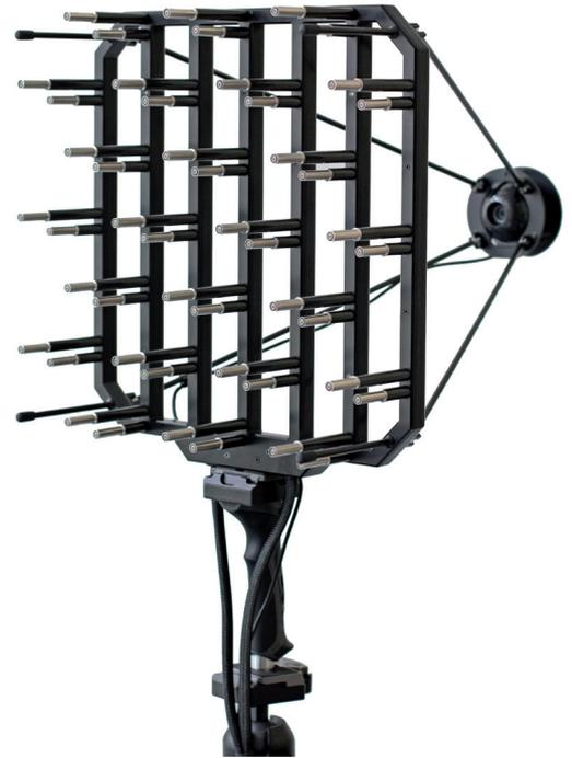
The design of the paddle allows for easy handling as it is lightweight and features cable bundling with one cable bundle holding 24 microphone channels.
