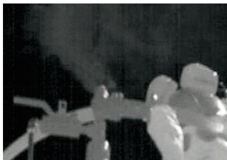
Thermal imaging with the GF306 can detect \text{SF}_6 leaks from plumbing or circuit breakers
