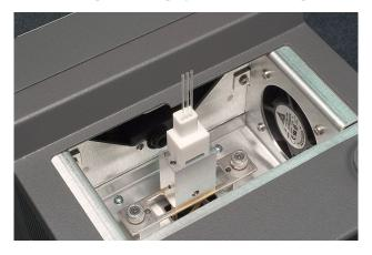
warm-up and cool-down cycling. Ramp rates from 0.1 °C/min. to 20 °C/min. (1-2-5 sequence) provide the flexibility needed for virtually any melt.
