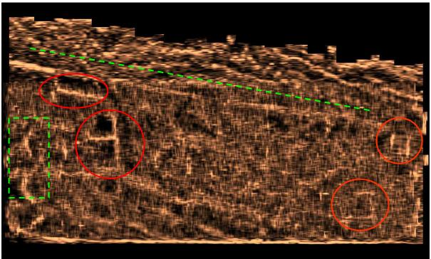
Depth: 0,7m. Looking at the tomography we easily detect some of the hidden targets (red circles). The green line represents an unsignaled pipe while the green box shows a couple of strong reflections of unknown origin. The final step of the survey is mapping our discoveries using a CAD interface.
