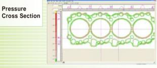
Pressure distribution on a line passing through a specified point is shown on a line graph
