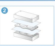
Insert Prescale between the pressure surfaces to be measured.
