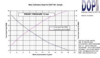
Sample mass calibration graph for DOP1100 Precision Thermal Generator offered as an option.
