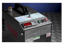
The vernier control is located immediately in front of the carry handle. Turning the vernier anticlockwise allows more oil into the heat exchanger and thus increasing aerosol output. The vernier is
