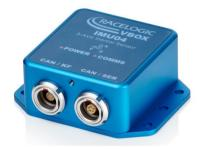
For accurate testing, even in areas where the view of the sky is obstructed, VBOX 3i v3 has the ability to gather additional information from an IMU (Inertial Measurement Unit – pictured left) and combine this with the GPS data in real-time to improve the quality of the parameters measured. To keep track of the attitude of the vehicle and greatly increase the velocity and position accuracy during periods when satellite visibility is poor, the IMU uses three accelerometers and gyros.
