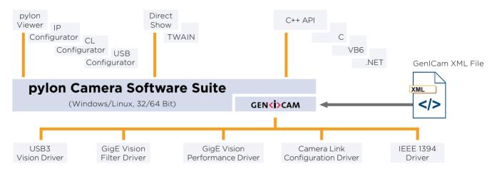
The architecture of the pylon Camera Software Suite is based on GenlCam Technology, which offers you easy access to the newest camera models and the latest features. Changes to an existing camera device in your application essentially become a plug-and-play process.
