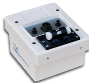
The TR900 antenna is designed for applications requiring higher penetration depth (up to 1 meter), for use in void detection, concrete thickness assessment and locating rebars.
