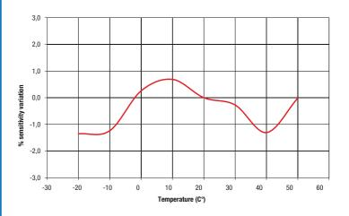
Graph1:% change of the sensitivity of the pyranometer LP PYRA 10 compared to the sensitivity at 20 ° C in the temperature range between -20 and 50 ° C.
