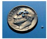
Micromachined Tilt Sensor Element
