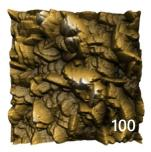
Consecutive unattended imaging of a TipCheck sample with CleanDrive excitation. After 100 images no noticeable change in the tip curvature could be observed. Image size: 1 µm. Z-height: 90 nm.
