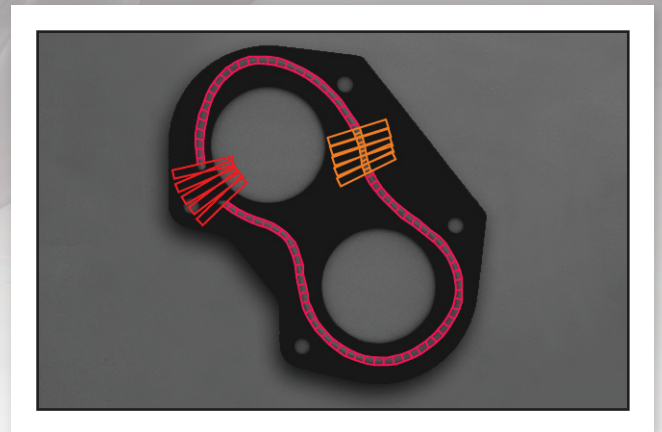
MIL Bead Inspection
