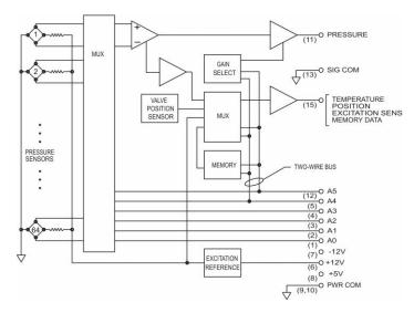
pressure measurements to the DTC System. Utilizing the calibration data within the EEPROM, the DTC System compensates for temperature changes to the sensors in real time reducing thermal error by a factor of 20 over conventional scanners. The ESP scanners also incorporate a hall effect sensor, which is used to indicate the position of the calibration manifold. This position information can be transferred to the system upon command.
