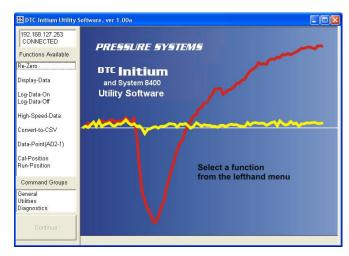
Utility routines include protected scanner EEPROM communication to enable stored data to be evaluated or manipulated as well as system firmware update using downloads offered at no charge from our website.
