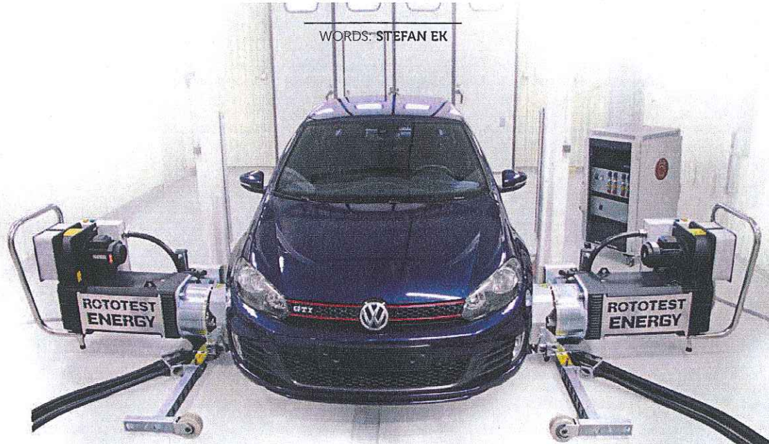
A typical 2WD setup of a Rototest Energy system
