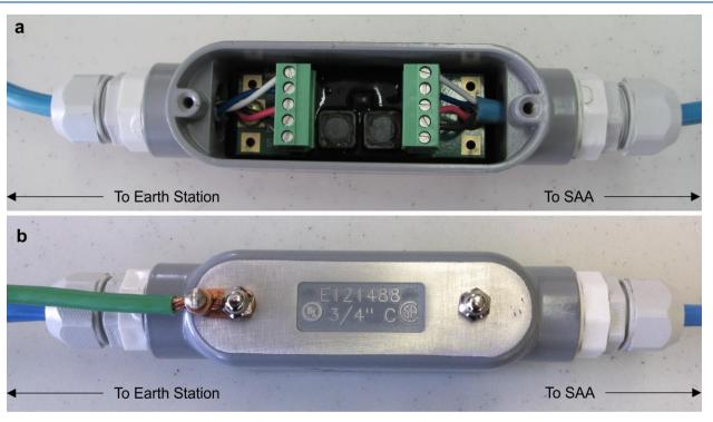
Figure 2.5 Fully wired SAASPD. a) Potting has not yet been done. b) Potting is done and ground wire is attached.
