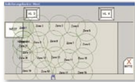
The waste bunker surface is divided in zones. The ThermoVision™ A40 checks every zone subsequently.
