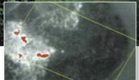
The infrared image shows hot-spots in the waste. This means a danger for spontaneous self-combustion and fire.
