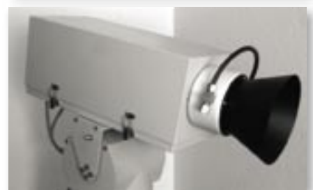
The ThermoVision™ A40 in its protective housing.
