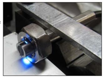
Plus and minus accept/reject tolerances can be set by comparing known good part voltages with known defective part voltages. Missing, shallow and/or damaged threads can be detected as they fall outside the accept/reject tolerance.
