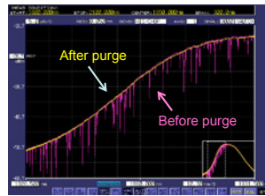
Effect of purging (dry-air, 1 hour) water vapor absorptions around 1900 nm
