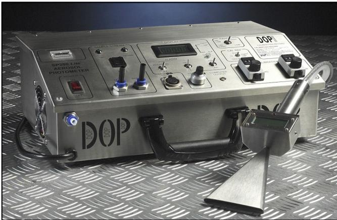
The DOP SOLUTIONS PHOTOMETER with the most advanced zero stability for testing HEPA and ULPA filters.
