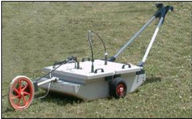
Separated transmitter and receiver antennas permit bi-static data collection (antennas can be spaced up to 1 meter apart).
