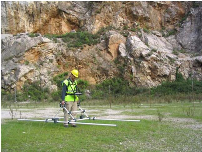
RIS Configuration with 25 MHz Unshielded Antenna- Acquisition Phase
