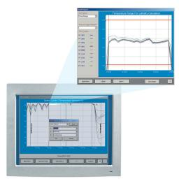
A powerful graphing utility within the system software greatly simplifies process analysis and reporting. Sliding vertical axes allow the operator to flag and define process transition points, eliminating unnecessary reporting and streamlining the review process.
