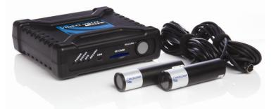
**Video VBOX Lite** takes the video captured from multiple waterproof cameras and combines it with a customisable graphic overlay, streaming the resulting video onto an SD card as a DVD quality MPEG4 file. A 10Hz GPS engine provides information such as circuit position, lap timing, speed (accurate to  $\pm 0.2$ km/h) and acceleration, whilst a single CAN channel can retrieve data such as RPM. CAN upgrades are also available to give a total of 2 or 4 channels.
