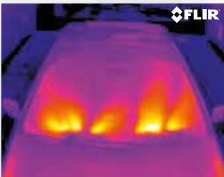
Inspection of car windscreen defrosting.
