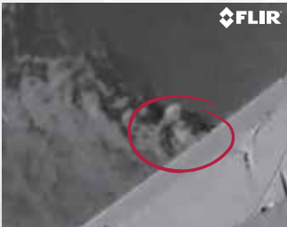
Captured gas leak from production site.
