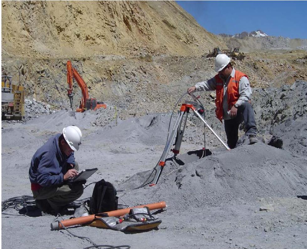
RIS Configuration with Bore Hole Antenna. Field Acquisition Phase
