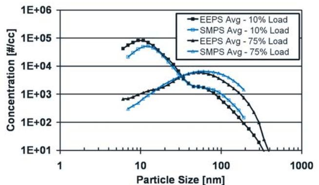
Figure 4. A comparison of SMPS and EEPS particle size data for a heavy-duty diesel engine.
