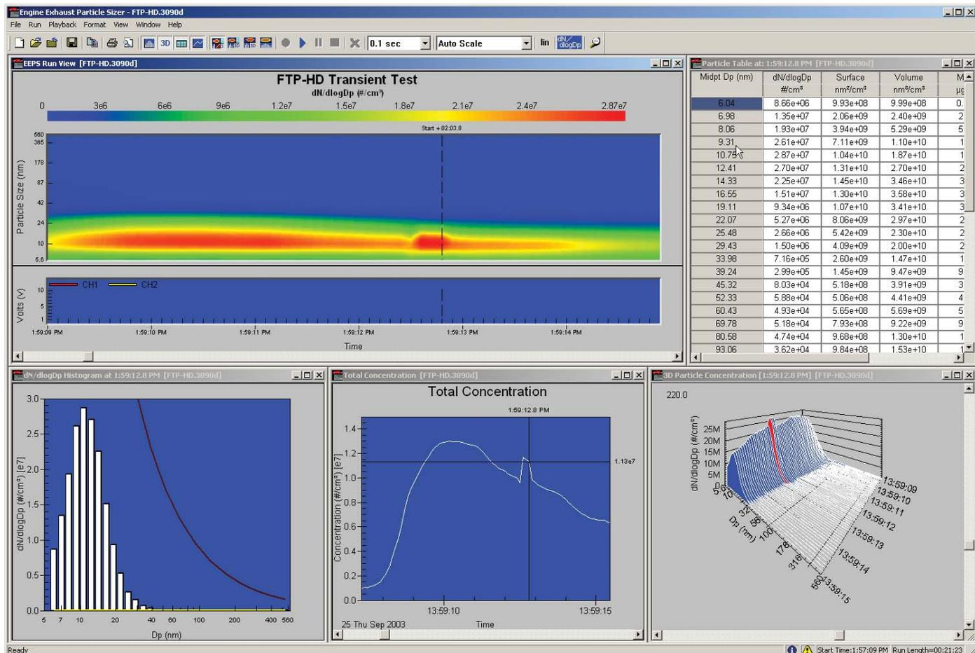
Figure 5. The EEPS software offers five main views of data. This screen depicts a large nucleation mode formed by deceleration during a transient test.
