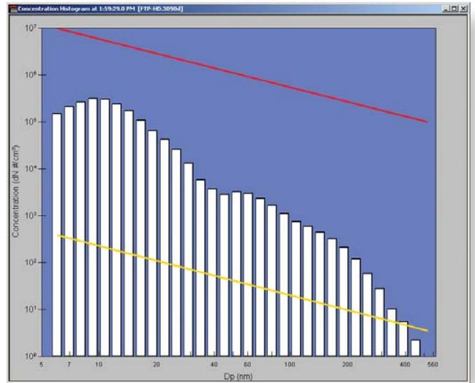
Figure 7. Histogram showing “in-range” concentration indicators (minimum in yellow; maximum in red). Log scale makes it easy to see nucleation and accumulation modes.
