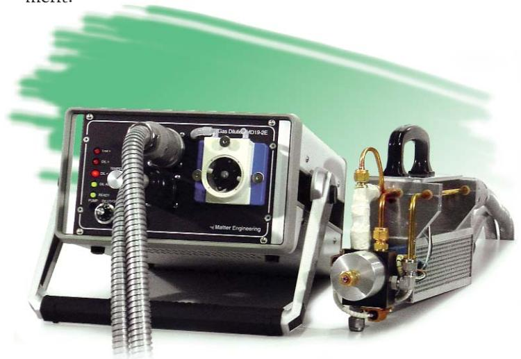
The Rotating Disk Thermodiluter accessory allows you to dilute the sample at the point of measurement. This preserves the size distribution and concentration so that particles are measured properly by the EEPS spectrometer. Dilution temperatures are selectable, enabling you to study volatile or semivolatile fractions.
