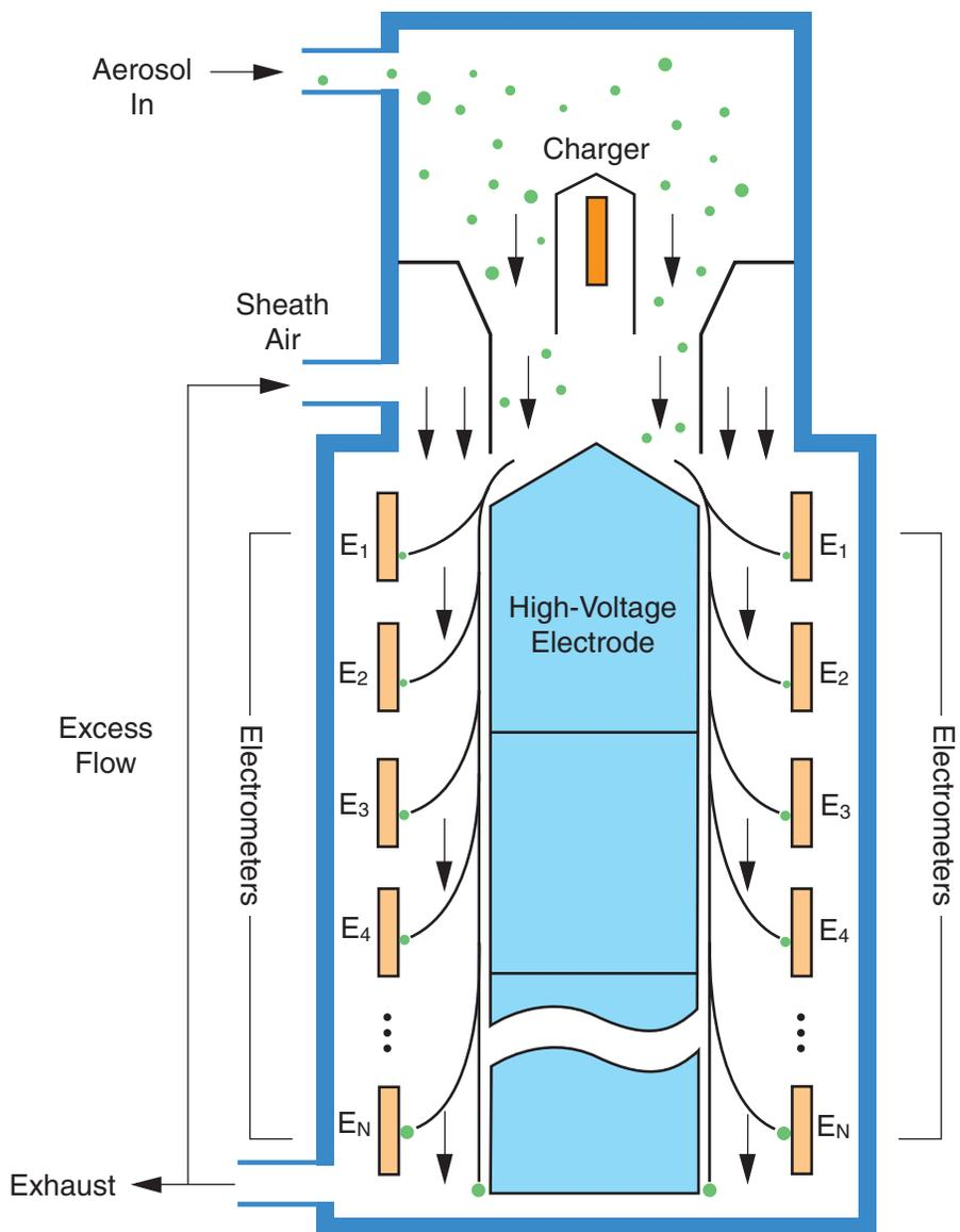
Figure 2. EEPS flow schematic
