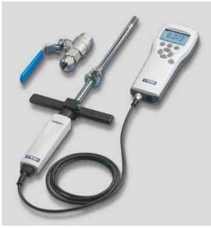
The MM70 is an ideal tool for the preventive maintenance of oil-filled systems. The water activity measurement indicates the margin to free water formation, which causes severe problems in lubrication systems.
