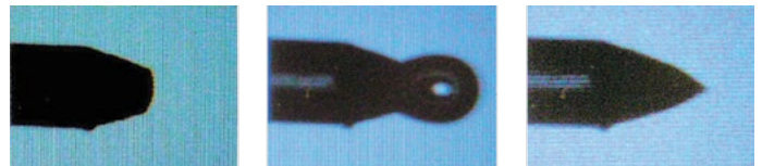
The 3482 electro spray produces particles down to 2 nm. The camera and viewing screen allows you to easily see the capillary tip during operation: (1) no liquid flow; (2) with liquid flow but no electric field; (3) with liquid flow and electric field (showing the formation of the Taylor cone).
