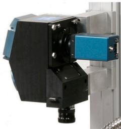
tivity and dynamic range. A design-optimized objective lens comes with each Starter Kit, providing excellent chromatic compensation and imaging results over the 250nm-600nm UV-VIS spectral range. The 28mm focal-length lens provided with the Hyperspec UV Starter Kit has been optimized for high resolution of UV wavelengths.
