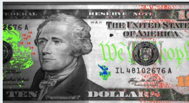
*Headwall's spectrometers provide a highly resolved means of determining the spectral makeup of any reflective material, including documents, currency, food products, and more.*
