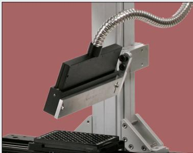
*Power-stabilized Pulsed Xenon UV and Quartz Tungsten Hologen (QTH) light sources.*
