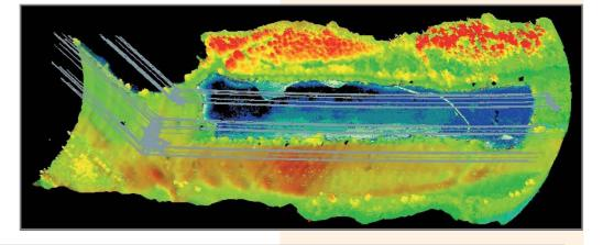
Cross section indicating targets above water level, subaqueous points, natural land targets and power lines.
