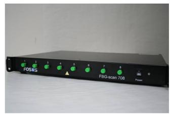
channel to be monitored can be selected by means of an optical switch. The internal Optical Spectrum Analyzer (OSA) is capable of performing FBG-peak detection with high accuracy. In addition, the optical spectrum of each input channel can be displayed. Both the updating rate of the OSA as well as the switching rate of the optical switch can be adjusted.
